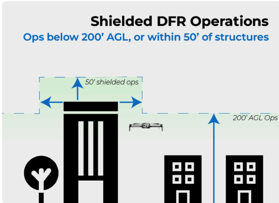
Operating at 200' AGL or within 50' of structures, a concept we called Shielded DFR Operations, in an urban environment provides a buffer between the drone and nearly all other aviation activities that are typically no lower than 500' AGL for their own safety, resulting in a safer operation by decreasing the likelihood of encountering low flying aircraft.
